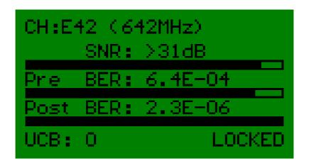
Hopefully, but not always, the digital readout; BER (bit error rate) and SNR (signal noice ratio) will correspond well with the analogue setting of the antenna.
