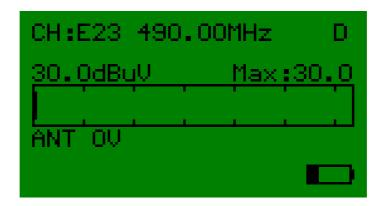
It is very easy to point an antenna towards a transmitter in this mode. The "maxhold function" (small bar in the big bar) will make it very accurate.
