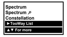
The Tooway functions and settings are available from the HD-TC8 sub menu as illustrated on the left. Within this group of menus it is possible to go back to the previous screen by using the left arrow key.
