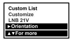
Once you have chosen the satellite you wish to find, enter the sub menu by pressing the **Off** button once. Then navigate down with the **On** button until the **Orientation** option is highlighted. Press the **right** arrow button to select this function.
