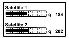
This screen shot indicates a locked condition where the quality figure is shown. Where possible we are looking to maximise the signal levels and the quality (number) indicator. Both satellites are being simultaneously measured.
