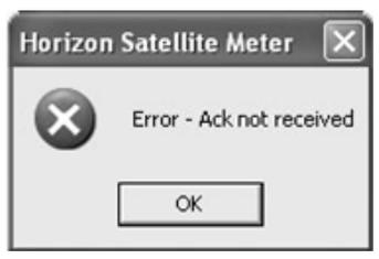
If you get this error message "Error – Ack Not Received". Check that the USB interface connection is correctly made and that the USB cable is undamaged.
