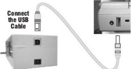
Wait for the HSDM USB / USB PLUS to display "Program Mode" (while establishing communication the display may flash and the sounder may beep. This is normal).
