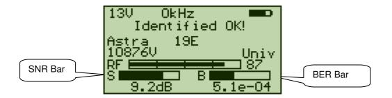
Once "Locked" on a signal, the satellite is confirmed with the MPEG data stream using the TSID and ONID (transport stream ID and Original Network ID) for the chosen transponder
