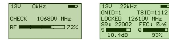
When a DVB-S signal has locked, the display changes to show the Symbol Rate and FEC. When the NIT information is available, it is also shown. (ONID is "Original" Network ID", and TSID is "Transport Stream ID")
