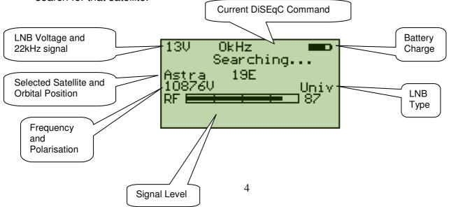
The signal level will increase on the signal bar if any satellite signal is detected. If the beeper is enabled, then the pitch of the beeper will increase with signal strength. Once the instrument locks on a satellite transponder, the display is changed to include SNR (signal to noise ratio) and BER (bit error rate) bars and numeric values.
